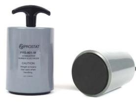
The PRS-801W is a precision milled resistance probe with conductive rubber pad for use with any resistance meter. Used in point to point and point to ground resistance testing of floors, worksurfaces, floor mats or any flat object, the PRS-801W produces repeatable measurements in accordance with ESD Association standards.
