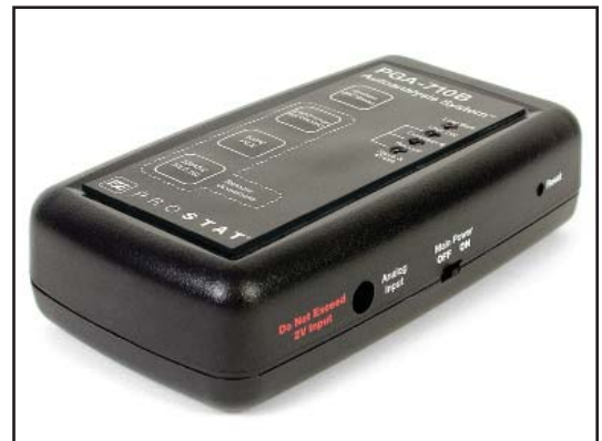
Figure 7: Main Power Battery Bus Slide Switch Isolates Battery during Storage
