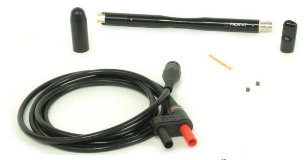
Accurately measures point-to-point resistance of small areas from  $0.90 \times 10^{12}$  ohms.
