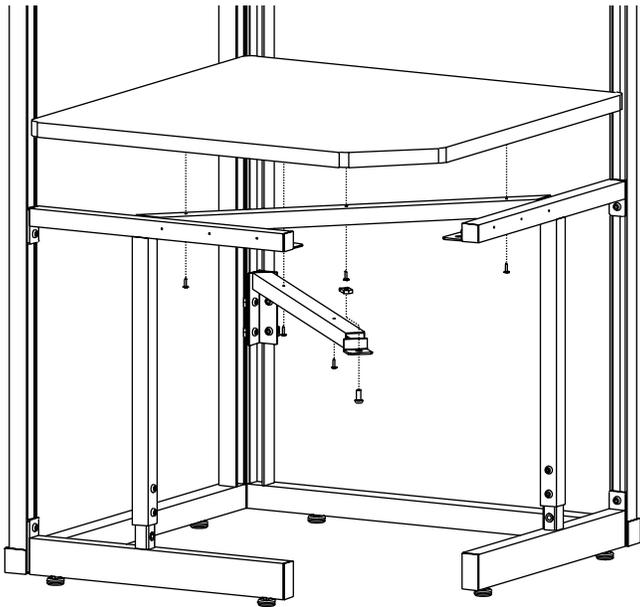
9. Place the laminate worksurface on top of the Worksurface Support Rail and ensure it is flush against the Frames and with the C-Legs on the sides. Face the seam of the T-mold edge toward the back. Attach the worksurface from underneath with wood screws.
