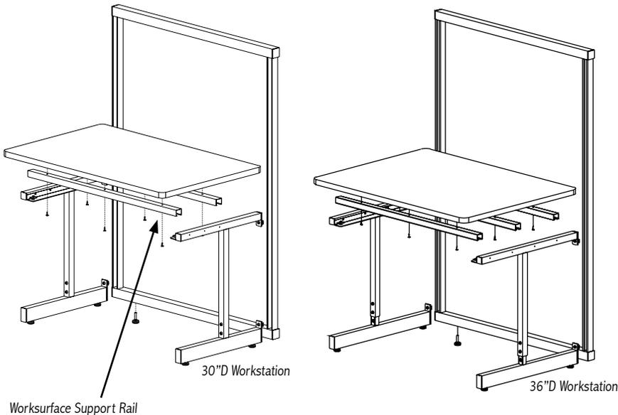
1. Insert two (2) Basic Bolts into pre-drilled holes determining height. Repeat for other C-Leg.
