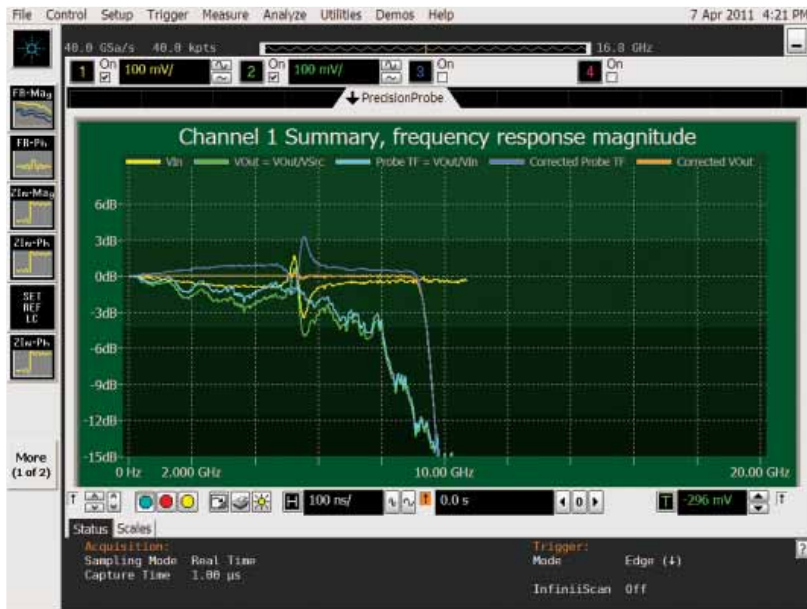
Figure 3. Frequency response of a probe as measured by PrecisionProbe.
