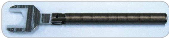
Figure 8. Straightened torque wrench
