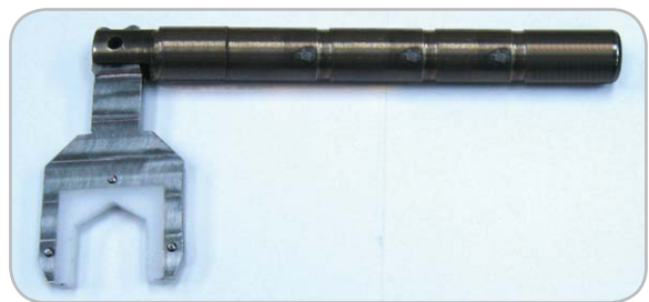
Figure 9. Bent torque wrench
