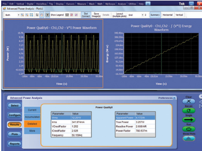
Figure 14. Power Quality results using DPOPWR.
