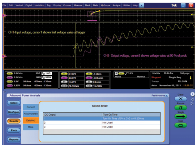
Figure 23. Turn-on Time results using DPOPWR.
