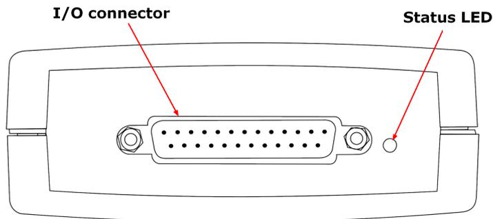
**I/O connector:** for the pin-numbering of the I/O connector, see [I/O connector pins](#). The Pico PP545 Small Terminal Board is specially designed to connect to this socket to allow you to make connections to individual wires easily without soldering. If you need to use a ribbon cable to connect your signals to this socket, use the shortest possible length to avoid introducing too much crosstalk between the signals.
