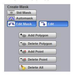
The **Edit Mask** function gives you access to a menu that allows you to construct a new mask, or edit an existing one, using the polygon method. The procedure of editing a mask function brings up a set of brief instructions on how to construct a mask.
