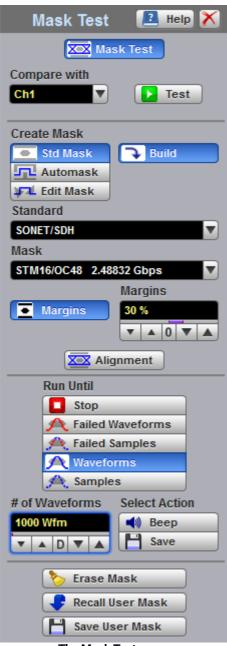
There are industry standards that define the parameters for electrical and optical waveforms. Mask testing is a process you can use to verify that the displayed waveform complies with an industry-standard waveform shape or with the user-defined mask.
