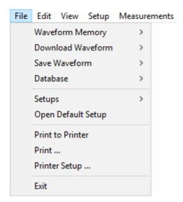
You may find it helpful to use this known operating condition when someone else has used the oscilloscope before you. If you accidentally press **Open Default Setup**, use **Undo** to return the oscilloscope to the operating condition it was in before **Open Default Setup** was pressed.
