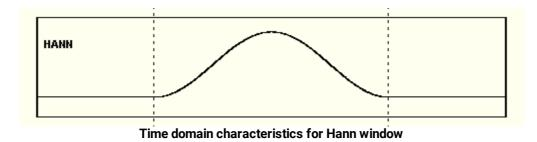
The **Hann** window is useful for frequency resolution and general-purpose use. Even though the overall shape of the time-domain signal has changed, the frequency content remains basically the same. The spectral line associated with the sinusoid spreads out a small amount in the frequency domain. It is good for resolving two frequencies that are close together or for making frequency measurements. The **Hann** window also improves amplitude accuracy.
