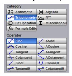
Below is a description of the twelve trigonometric operators. There are four standard trigonometric functions, four inverse trigonometric functions, and four hyperbolic functions.
