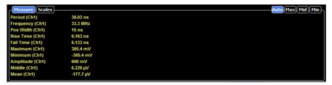
Measure tab with the results of ten automated parameter measurements
