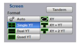
The **Format** menu determines how the instrument draws the waveforms on the display. The following formats are used in the PicoScope 9400 Series.
