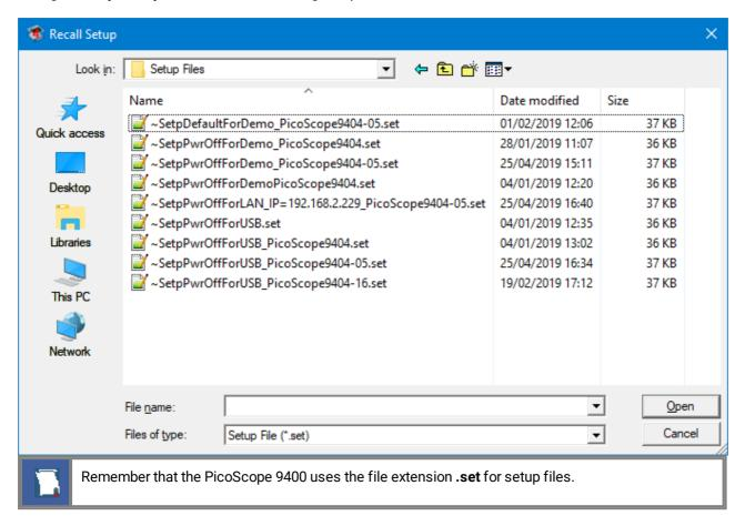
Recalling a setup replaces the current setup with the recalled setup. If you do not want to lose your current setup, save it to its own setup file for later recall before you recall the new setup.
