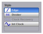
There are several different styles of trigger used in digitizing oscilloscopes. The PicoScope 9400 Series uses **Edge**, **Divided**, **Clock recovery**, **Internal clock** and **External Prescaler** styles.
