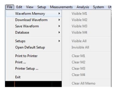
The **Download Waveform** submenu loads the selected file from a disk into one of the memories M1–M4. This submenu includes the following controls:
