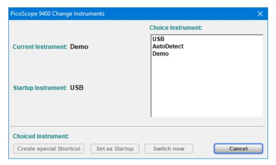
This dialog allows you select the instrument that should be assigned to the program. The following options can be used:
