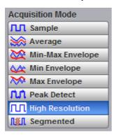
Acquisition Mode lets you choose how the oscilloscope will create points in the waveform record.
