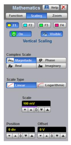
The Scaling menu for complex waveforms
