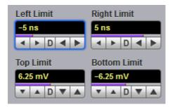
The **Left Limit, Right Limit, Top Limit** and **Bottom Limit variables** allow you to use the histogram limits to select a region of the database.
