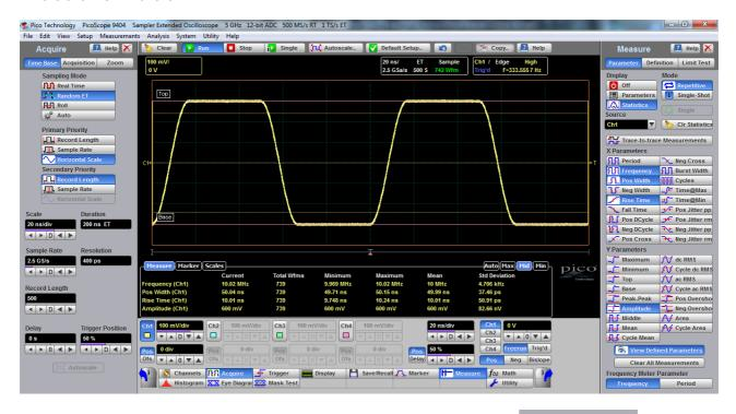
7. To take a measurement on another channel, select that channel from **Source** select the measurement.
