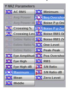
The list of **Y NRZ Eye Parameters** includes twenty-seven eye parameters.
