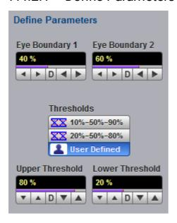
The **Define Parameters** menu sets the measurement points (boundaries and thresholds) where the automatic measurements are made. The menu influences the measurement algorithm by allowing you to use the standard measurement points, or customize the measurements with user-defined selections.
