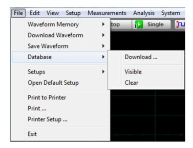
**Download** opens the Windows **Load Database** dialog and allows you to select a database file to recall from disk to Database Memory (**DB**).
