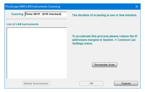
After the scan is finished, all found IP addresses will be displayed in the **List of LAN Instruments**. To confirm the scanning results, click **OK**.
