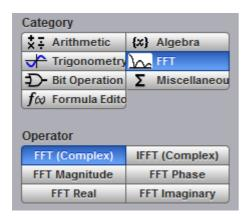
The **FFT** menu allows you to control the operation of the FFT (Fast Fourier Transform), including spectrum selection and display, and also a choice of six FFT windowing functions. Refer to the **Scaling** menu for formatting a spectrum with different complex scales, and also for scaling and positioning it.
