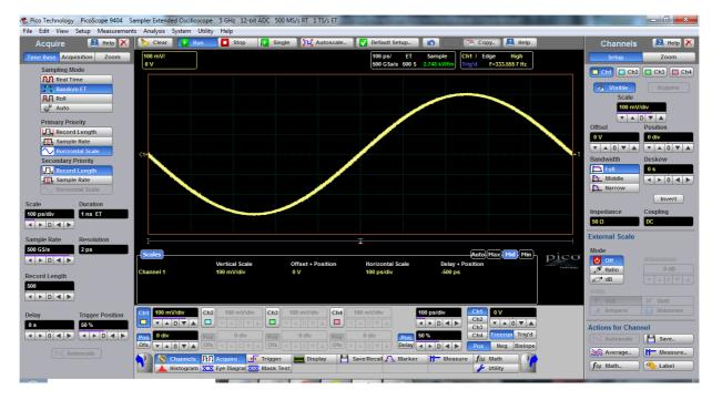
5. Use waveform <u>averaging</u> if level of noise or jitter exceeds what is acceptable for your measurements.
