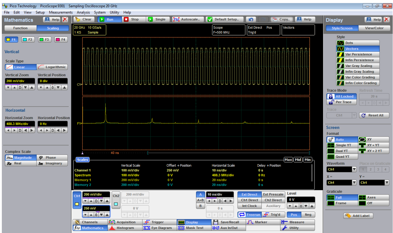
Spectrum Magnitude of 500 MHz pulse waveform
