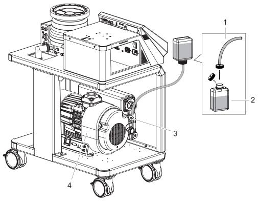
Fig. 20: Filling up with operating fluid – example SmartVane
