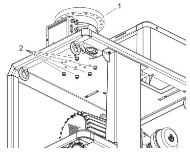
Fig. 61: Removing turbopump – free-standing model
