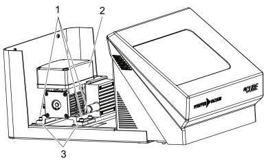
Fig. 67: Installing backing pump – desktop model
