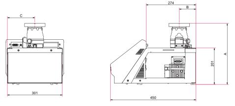
Fig. 71: Dimensions HiCube Neo – desktop model Dimensions in mm
