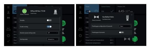
Fig. 32: Parameters in the vacuum monitor
