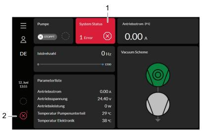
Fig. 69: Example of an error message on the dashboard
