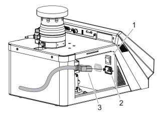
Fig. 58: Removing electrical connections
