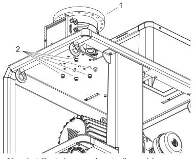
Fig. 64: Installing turbopump – free-standing model
