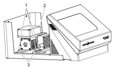
Fig. 65: Removing backing pump – desktop model
