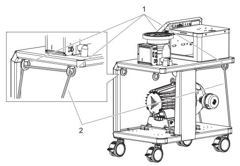
Fig. 9: Anchoring the free-standing model
