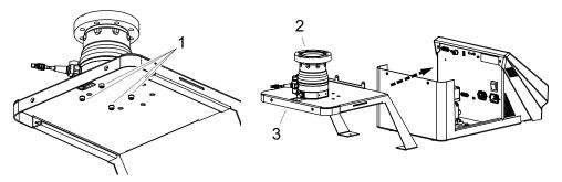
Fig. 62: Installing turbopump – desktop model
