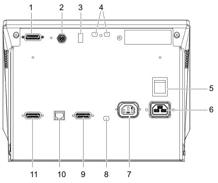
Fig. 24: Overview of all interfaces and connectors
