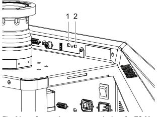
Fig. 21: Connecting accessory devices for TC 80 and TC 110
