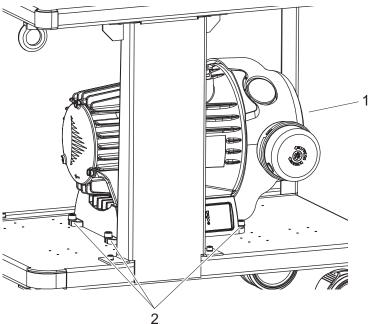
Fig. 66: Removing backing pump example – HiScroll
