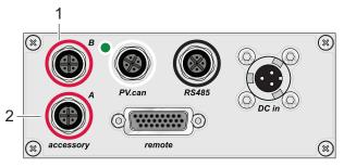
Fig. 22: Connecting accessory devices for TC 400
