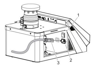
Fig. 23: Connecting to mains power supply
