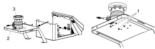
Fig. 60: Removing turbopump – desktop model
