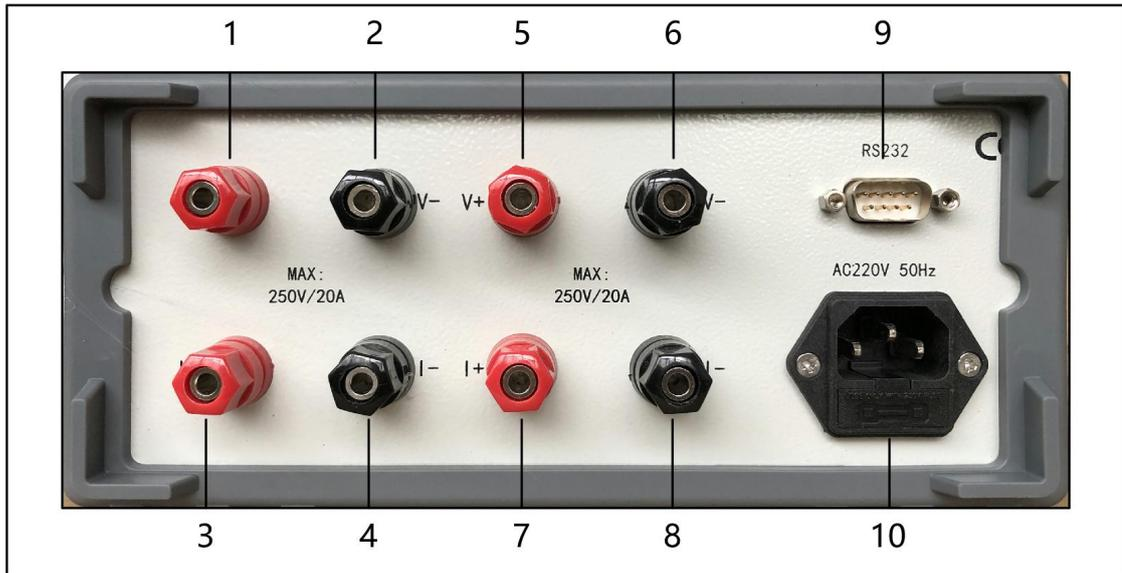
As shown in the above figure: connect the channel 1 voltage input into the terminal 5-6 (pay attention to distinguish L/N), connect the channel 1 load to the terminal 7-8 (pay attention to distinction L/N), then Channel 1 wire connection is finished.
