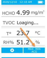
Now press the left key repeatedly to display the desired measurement function. Use the right key to pause and resume the evaluation. Press the back key to return to measuring mode.
