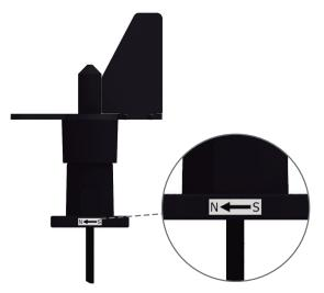
To orientate the vane north, the vane edge must be orientated north as shown in the picture.
