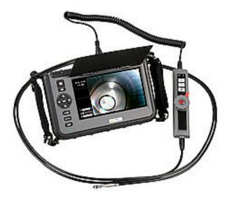
Different cables can be connected to the inspection camera / Image and video recordings / large 7" LCD display for precise viewing / Recording on SD card / Pictures rotatable by 360° (90° steps) / Bright LEDs on the camera head / Digital zoom
