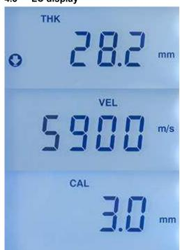
THK (thickness): material thickness measurement
