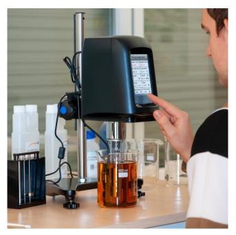
Precise viscometer with 5" touchscreen / temperature sensor / laboratory stand / measuring range up to 2,000,000 cP / 4 different attachable spindles / for measuring the viscosity of liquids / RS232 interface
