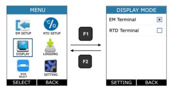
There is mainly three RUN Display Mode possible in this device. And this mode can be selected from the above Page. What information to be shown in each RUN Display Mode can be defined by this page.
