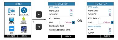
This page contains parameters related to RTD like RTD Mode Type, RTD select, Unit, RTD Source Mode etc. The Description of the Parameters appear on this page is given below.
