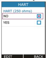
Select YES to add a Series resistor ( $250\Omega$ ) into the mA circuit. You can then use this instrument together with a HART® communicator to set up and calibrate HART® devices. This option is applicable for mA(24V) Read Power Input Type Only.
