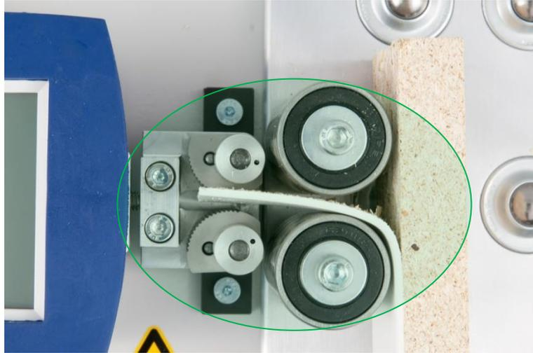
The measurement can be started. The sample was inserted correctly.
