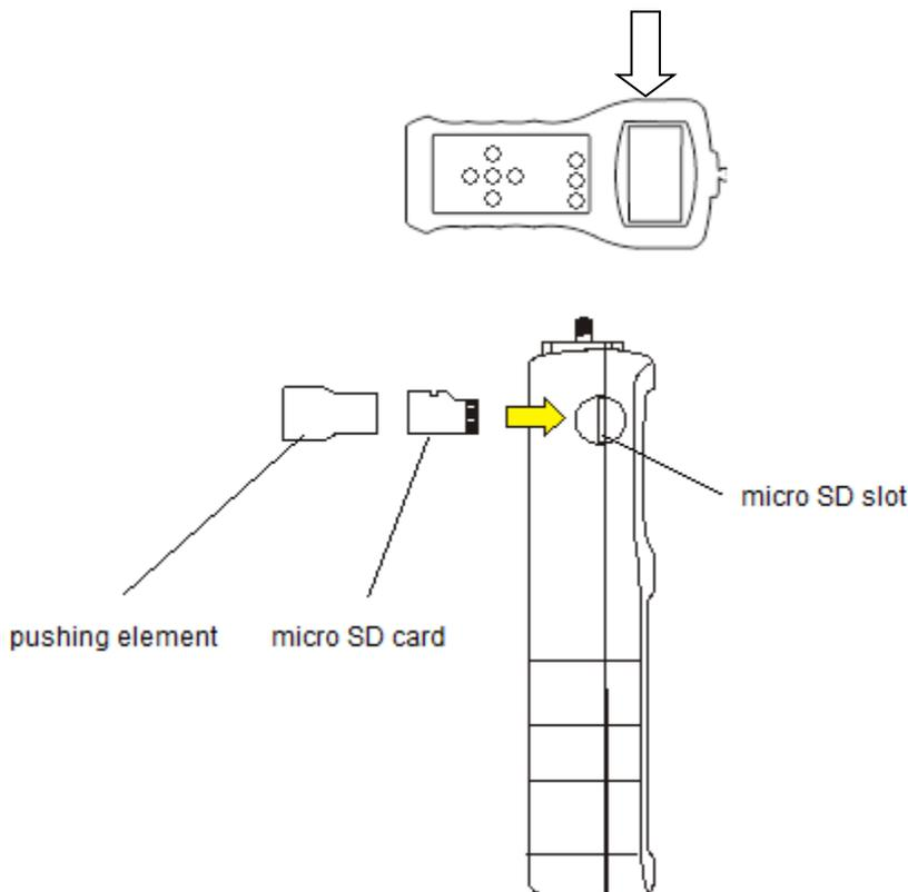
To insert a microSD card, turn off the device and put the card in the slot. Use the pushing element to push the SD card in, until it snaps into place. Now turn on the device. An SD symbol should appear in the display. To remove the SD card, turn off the device once again and use the pushing element to push the card further in, until the holding mechanism is released.
