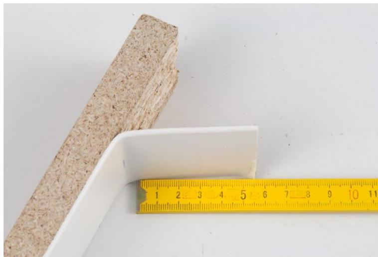
4. Insert the sample into the PCE-PST 1 as seen in the following image. Make sure the peeled-off stripe is not too short or too long.
