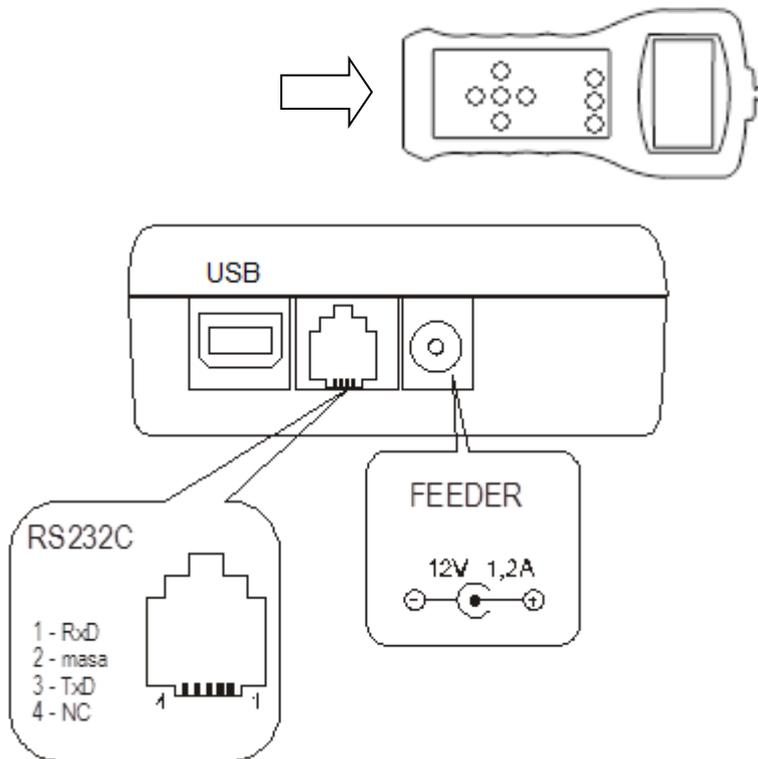
On the bottom of the force gauge you can find an USB and a RS-232C interface, as well as a connector for power supply.
