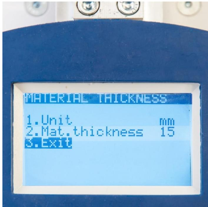
Here you can set the material thickness and the unit in which it is displayed. Select the desired option by using the „PEAK ▲“ and „MENU ▼“ keys and press „ENTER ►0◀“. To change the unit, use the „MEM ◀“ and „PRINT ▶“ keys. To change the thickness, select a digit by using „MEM ◀“ und „PRINT ▶“ and increase or decrease it by using „PEAK ▲“ and „MENU ▼“. Press „ENTER ►0◀“ afterwards to confirm.
