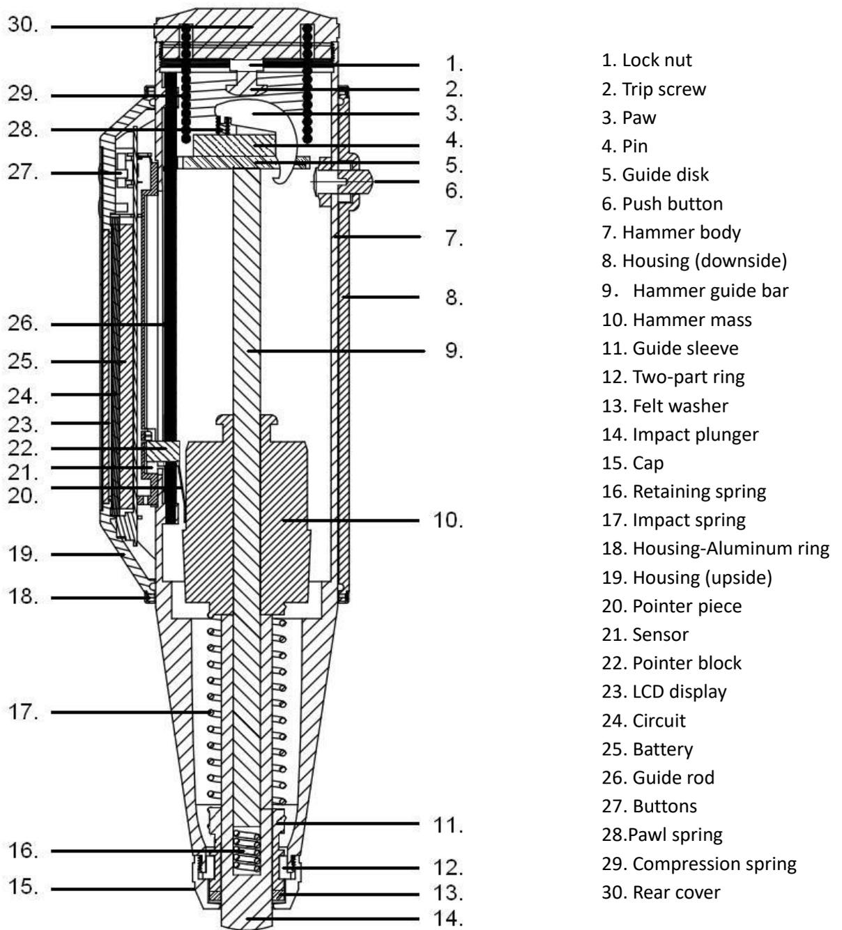
Structure of Concrete Hammer
