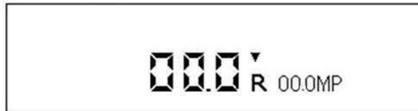
Measuring interface in 30% power consumption, in this mode, the instrument could work 13-16 hours after fully charging.
