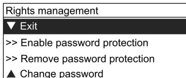
In this menu, user can enable, disable and change password for this instrument. After enable and set password, the password needs to be input for Re-view data, Upper-Lower limit setup and rights management.
