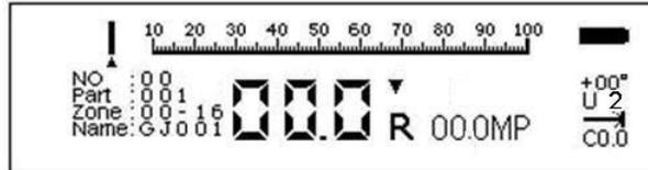
Measuring interface in 60% power consumption, in this mode, the instrument could work 10-13 hours after fully charging.
