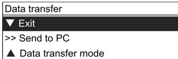
Before creating communication between instrument and PC, use USB cable to connect PC and the instrument, then enter Data transfer menu to select Data transfer mode. Cable for USB connection, Bluetooth for Bluetooth wireless connection (option). Off to disable Bluetooth connection.
