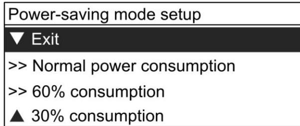
In this menu, there are 3 kinds of power consumption modes for choosing. Measuring interface in normal power consumption, in this mode, the instrument could work 8-10 hours after fully charging.
