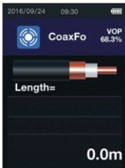
Measuring mode for coaxial cables and cables connected to the meter with a measuring adaptor
