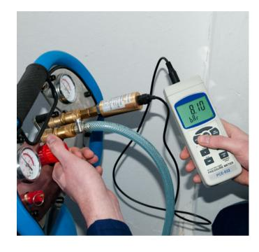
PCE-932 is an easy-to-use, digital, handheld device for high pressure measurement in hydraulic and compressor systems, pumps, tanks and silos in chemical, manufacturing, plastics and HVAC industries. This portable pressure measuring device can be connected to pressure sensors with ranges up to 400 bar (each with a 1.2 m connecting cable).
