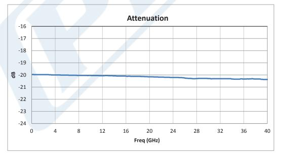
Click the following link (or enter part number in "SEARCH" on website) to obtain additional part information including price, inventory and certifications: 20 dB Fixed Attenuator, 2.92mm Male to 2.92mm Female Passivated Stainless Steel Body Rated to 2 Watts Up to 40 GHz PE7395-20
