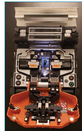
Figure 4: Fusion Splicer shown open, Fiber Sheaths closed.
