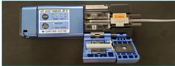
Figure 7: Removing the jacket from the fiber.
