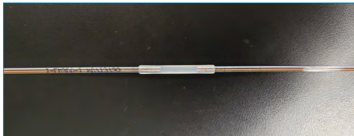
Figure 1: 12-ribbon fiber, post arc procedure.
