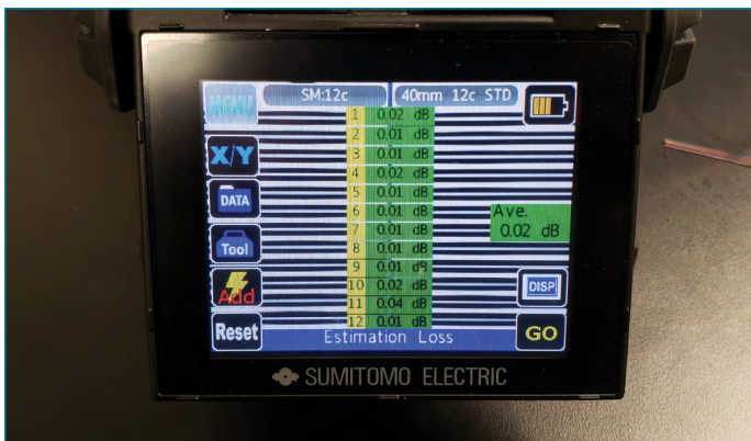
Figure 13: Image of completed arc process on the LCD screen.
