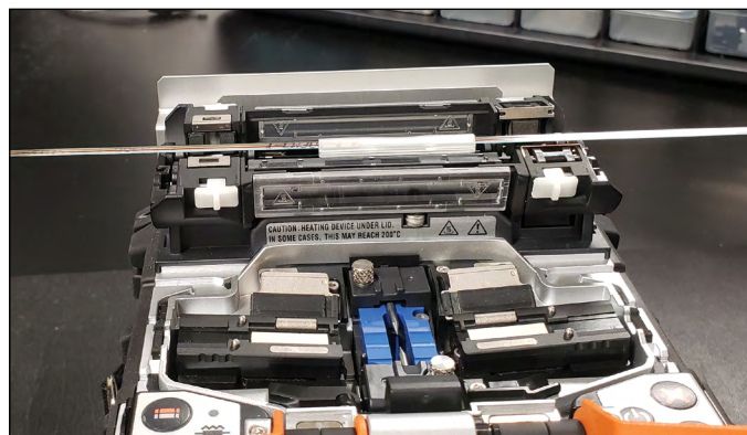
Figure 16: Spliced Fiber with splicing sleeve in place, being laid into Oven 1.
