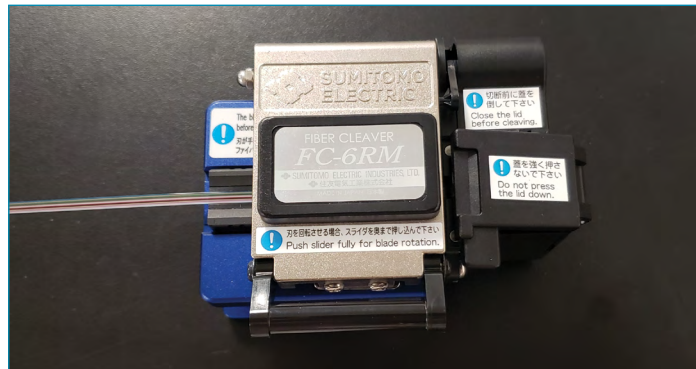
Figure 9: Cleaving the bare fiber(s).
