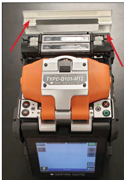
Figure 18: View of dual cooling trays.
