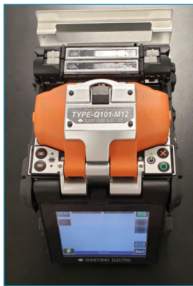
Ribbon Fiber Fusion Splicer Example – Sumitomo Type-Q101-M12 Mass Fusion Splicer
