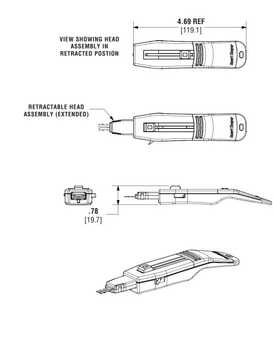
Dimensions are in inches. [Dimensions in brackets are metric].
