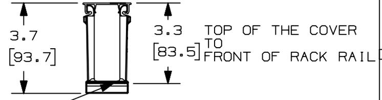
SURFACE IN CONTACT WITH FRONT OF THE RACK RAIL
