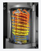
The Inductive Convection Heater pre-heats the air in a cyclonic fashion around the induction coil before entering the inner chamber, where the air is instantly heated to the target temperature. The low thermal mass design then allows the coil to cool down at a faster rate, consistently yielding high quality solder joints.
