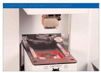
PBGA being held by Vacuum pik during Alignment procedure
