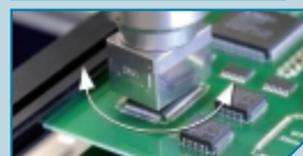
PACE UNIQUE FEATURE (Twist) Simple coplanarity adjustment allows for extract nozzle adjustment, much better than fixed head systems.
