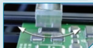
PACE UNIQUE FEATURE Simple coplanarity adjustment allows for extract nozzle adjustment, much better than fixed head systems.
