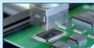
Fast and repeatable nozzle height adjustment with mechanical stop for consistency of process.
