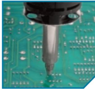
▲ SX-80 Desoldering Thru-hole Solder Joint
