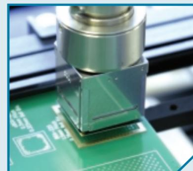
BGA alignment is easy with PACE's proven template alignment method.
