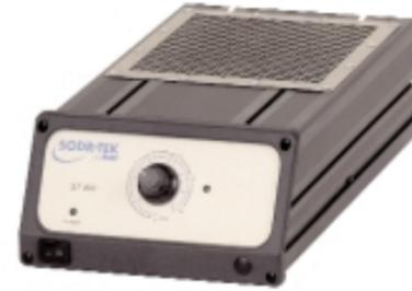
The ST 400 is an analog, closed loop, temperature controlled radiant 400 W pre heater. The heating area is 140mm x 140mm (5.5" x 5.5"). This preheater is ideal for heavy PCBs and for area array applications as the medium wave IR delivers the most penetrating and even heating available. The ST 400 can be used as a stand-alone unit with either the ST 525/ST 550 PCB holder or can be used with the ST 300, ST 325, or ST 350.
