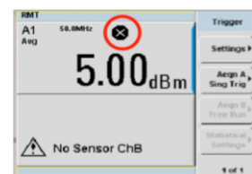
Figure 2. Triggering mode in Single Trigger
