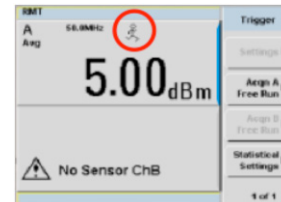
Figure 1. Triggering mode in Free Run
