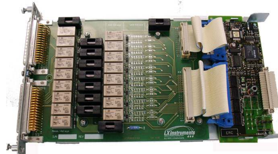
Figure 2. Keysight 34959A breadboard module with LXinstruments circuitry.
