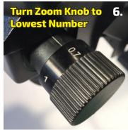
**NOTE:** For trinocular microscope models, keep the microscope body set to its **lowest zoom setting**, and twist the knurled rubber ring on the CCD adapter until what you see is in focus. Verify focus by zooming through the entire magnification range, and adjust slightly if required. This focus adjustment should not need to be completed again unless you remove the camera.
