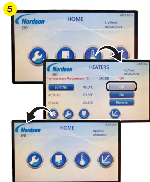
Switching OFF heater control and returning to the HOME screen
