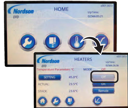
Switching OFF heater control
