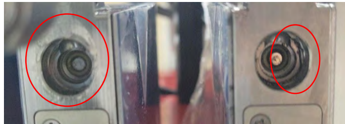
Examples of Pμlse valve actuators with UV adhesive contamination in the push-rod cavity
