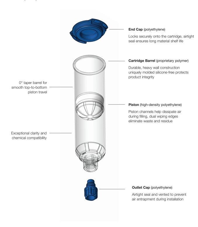
Optimum cartridges are molded from a strong, clear FDA- and RoHS-compliant polymer, with ZeroDraft walls that maintain consistent internal diameters for smooth piston travel.
