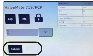
Main screen when the lock / unlock function is enabled and the system is locked; a password is required
