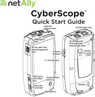
The CyberScope<sup>®</sup> is a rugged, handheld cyber security scanner. The multifunction tools and various applications allow comprehensive site security surveying, analysis, and reporting for your on-premises site networks.
