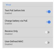
Test PoE before Link: By default, an AutoTest Wired Profile performs the Link test before the PoE test can complete. Enable this setting to make your LinkRunner complete the PoE test before the Link test. Enabling this setting forces PoE negotiation to be completed before establishing link, improving compatibility with some switches.
