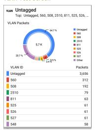
The VLAN test screen displays the real-time traffic the LinkRunner detects on the top VLANs. Up to nine VLANs with the highest traffic are displayed as colored portions of the pie chart.
