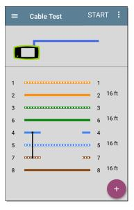
This unterminated cable test image shows a shorted cable between pins 4, 5, and 7.
