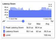
Latency (Up/Down): Latency is the amount of time it takes for a packet to go from the source to the endpoint or from the endpoint to the source (in milliseconds). Latency is calculated by averaging the thousands of latencies measured during each interval. The one-way latency measurements are actually round trip measurements, divided by two.
