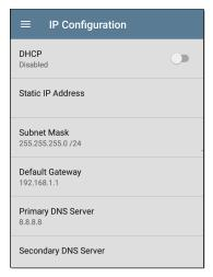
The Static IP address fields for **Subnet Mask, Default Gateway**, and **Primary** and **Secondary DNS Servers** only appear if DHCP is disabled. Tap each field to open a pop-up number pad and enter the static addresses as needed. Tap **OK** to save your entries.
