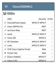
On the SSIDs screen, each SSID is shown with its Security type(s) and any VLANs. SSIDs with a checkmark to the left are enabled, and those with an × are disabled.
