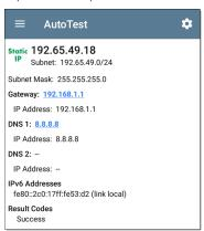
The Static IP test screen displays the configured addresses.
