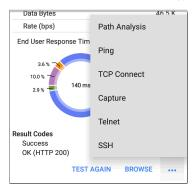
Tap blue links or the blue action overflow icon ••• at the bottom of the test results screens to run the HTTP TEST AGAIN, open another testing app, or Browse to the target address in your web browser.
