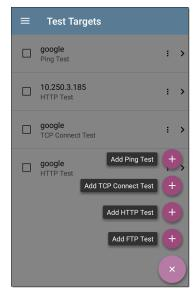
Tap any target test name to open that test's settings. You can then enter a custom test name, target address, or thresholds. For more information on settings, see:
