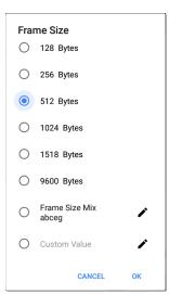
Selecting Frame Size Mix creates traffic with variable frame size patterns, generated in a repeating sequence. Tap the edit icon to revise the frame size pattern.
