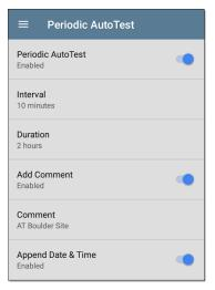
Tap the **Periodic AutoTest** field to enable, and adjust the settings below as needed.
