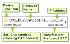
The lower left field displays the characteristic by which the Discovery list is currently sorted. In the image above, the list is sorted by MAC address. See Discovery Sorts in this topic for more about sorting.
