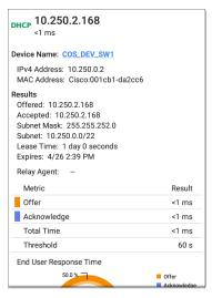
**Device Name**: The discovered name of the DHCP Server, or, if no name could be discovered, the IP address
