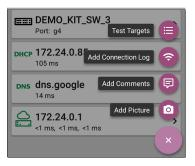
The Test Targets screen lists all of the defined and saved Test Targets. Checked boxes indicate the Test Targets that are enabled in the current Profile. Remember, Test Targets can be added to and used in any number of Wired Profiles.
