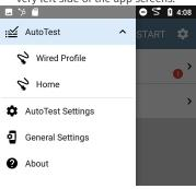
As an example, the AutoTest navigation drawer (above) provides access to the enabled AutoTest profiles, AutoTest Settings, General Settings, and the About screen.
