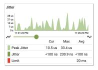
Jitter (Up/Down): Jitter is a measure of the variation in frame-to-frame latency in milliseconds
