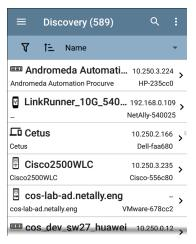
Like in AutoTest and other LinkRunner screens, the icons in Discovery change color to indicate a Warning or Failure condition. Discovery also displays device icons in Blue to indicate Problem-related information that does not constitute a warning or failure, and **Green** to indicate that a previous Problem has been resolved. (See the Problem Settings to adjust enabled Problems and thresholds.)
