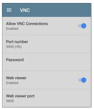
**Allow VNC Connections**: (Disabled by default.) Tap the toggle button to enable remote
