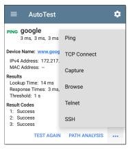
Tap blue links or the blue action overflow icon ••• at the bottom of the test results screens to run the Ping TEST AGAIN, open another testing app, Browse to the Ping target address in your web browser, or start a Telnet or SSH session.
