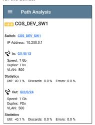
A Layer 2 Details screen displays the device name and IP address at the top.
