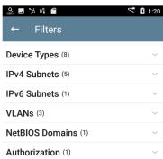
The Filters screen displays the number of devices or domains discovered for each category. Tap a category name to select filters by checking the boxes. The main Discovery screen shows only those devices or IDs that fall under your chosen filter parameters.
