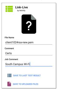
Enter any Comments you would like attached to your file. c. Select SAVE TO LAST TEST RESULT or SAVE TO UPLOADED FILES. Your files are then uploaded and viewable on Link-Live.com. (The SAVE TO LAST TEST RESULT option attaches the image to your most recently run AutoTest, Performance, iPerf, or Cable Test results on Link-Live.com.)
