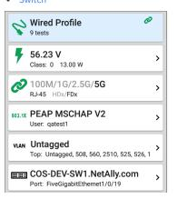
The 802.1X card only appears if the **802.1X** setting is enabled for the Wired Profile.
