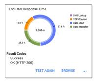
**End User Response Time**: Pie chart of the times for each phase of the test (DNS, Lookup, TCP Connect, Data Start, and Data Transfer)
