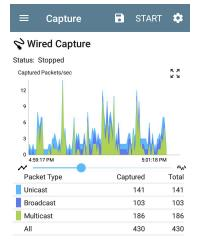
To pan, or move backward and forward in time, touch and drag (swipe) left and right on each graph.
