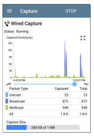
The graph plots the type and number of packets being captured while the capture is running and includes Unicast, Broadcast, and Multicast packet types.
