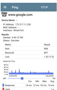
The graphs update in real time and then save and display data for up to 24 hours (depending on test type and/or link status).
