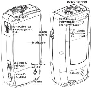
The LinkRunner® 10G is a rugged, hand-held tool for testing and analyzing wired copper and fiber Ethernet networks. This Multi-Gig Network Tester features applications developed by NetAlly for wired network measurement and validation.
