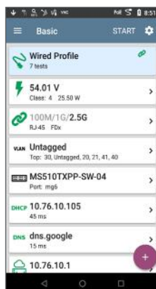
NBASE-T network with VLAN and 802.1x authentication
