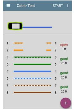
**NOTE:** Open/un-terminated cables with crossovers will display as "good" because LRAT cannot detect crossovers in un-terminated cables.
