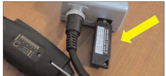
The program Key **cannot** be used with NF-Series Standard Plus Models & Angle & Auto Reverse Models.
