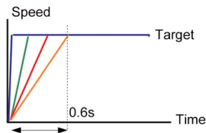
The Soft Start button is “wrap around” button meaning you can toggle through the settings continuously by pressing the button (OFF - 0.2s-0.4s-0.6s).
