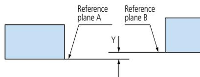
d. Angle between reference planes A and B:  $\theta_y$  (angle)
