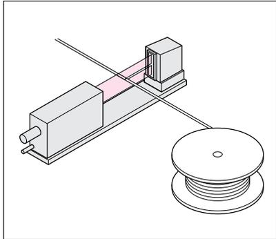
Outer diameter of opaque or transparent cylinders
