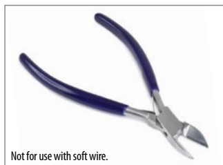
#89117 Hard Wire-Cutting Plier with Carbide Jaw Inserts Got a hard wire cutting job? Either you can get this plier or plan on trashing anything else! Carbide inserts at the jaws' cutting edge bite through music wire up to 13 gauge (.031") and other spring-type wire up to .048" with ease. Other quality features include box joint fulcrum for exceptional leverage without straining and spring return action. 7" long overall with 1" nose. $29.95
