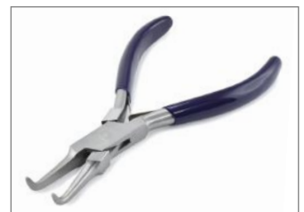
#89119 90° Bent Nose Plier This clever variation of needle nose pliers features non-serrated tapered jaws that are bent at a 90° angle, 3/8" from the tip. This allows the jaws to grip in tight spaces and at angles which ordinary pliers can't. Useful for many applications including soldering, wire and jewelry work, model building and more. Box joint construction with leaf spring return. 5-1/2" long. $9.95
