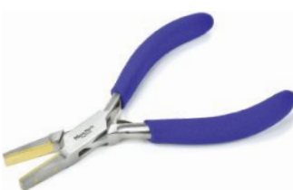
#90144 Non-Marring Brass Jaw Flat-Nosed Plier This non-marring brass-lined plier offers a much firmer platform than the nylon-lined type for superior bending, and the flat, half-hard brass won't damage the material being formed. The 1/4" wide by 7/8" long brass jaw linings have tips that close to zero. Made from stainless steel, this 5-3/4"-long plier features leaf springs, box joint construction, and super-comfortable foam grip handles. $15.95
