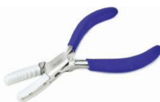
#90145 Non-Marring Nylon Jaw Tube and Rod Plier Nylon jaw inserts eliminate marks and nicks when working with wire, rods and tubing. Designed with mating semi-circular indentations in each jaw side, the plier safely holds #6 - #16 gauge wire and tubing, and rods from .050" to .160" dia. Tips close to zero to grab even thinner material. 6-1/2"-long stainless steel plier features leaf springs, box joint construction, and foam grip handles. Includes an extra pair of nylon jaw linings and screws. $15.95
