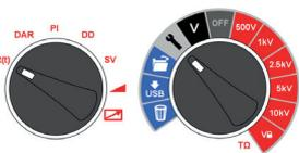
A timed test IR(t) will automatically terminate an insulation test after a preset time. Default timer is set to 1 minute and is adjustable within the settings function. This is a useful feature which saves the user watching the display for the full duration of the test and the possibility of missing the 1 minute reading.
