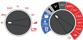
To set the user defined lock voltage  $V_{\text{lock}}$ , turn the central rotary switch to settings and the mode switch to IR. The preset voltage will flash and can be changed using the up/down buttons. When the required maximum voltage is displayed, press the OK button to save the setting. This setting will remain until it is reset.
