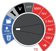
Downloading data function is selected by switching to the 'download via USB' icon on the central rotary switch. Before starting a download a USB PC-to-device cable must be connected between a PC and the USB port on the instrument, or alternatively a Bluetooth® connection setup to a suitably enabled PC or similar device.
