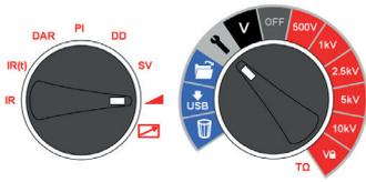
The ramp voltage test is an overvoltage test similar to the SV test but with many very small steps. The slow continuous voltage ramp is less likely to result in unpredictable damage to the insulation than the rapid step increases employed in SV test.
