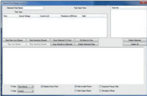
Import/Live Stream Control application enables capture of live streaming data directly by activating the Start New Live Streaming function. Results are recorded once a second for the duration of the test
