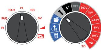
DAR and PI tests are measurements of resistance over time expressed as a ratio of resistance at time t2 divided by resistance at time t1. The assumption is that insulation temperature does not vary widely over the duration of the test so the resulting DAR and/or PI value are temperature independent. Testing should be done at or below 40 °C, 104 °F for this assumption to hold.
