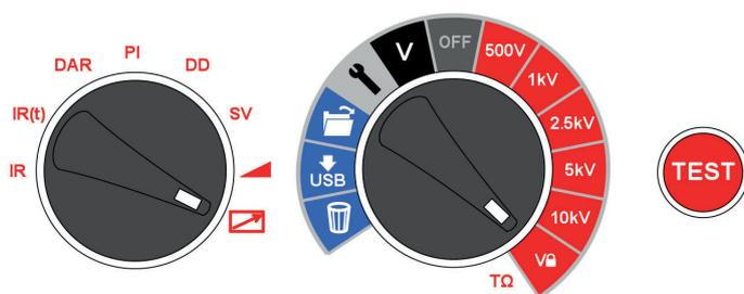
Instrument controls are simple to operate. The central rotary switch incorporates the OFF position. The left hand rotary switch selects insulation test type. The TEST button starts and stops a test. Image depicts instrument setup for Remote Control mode.
