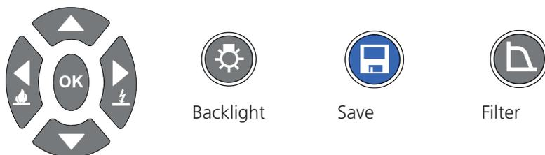
Four arrow buttons + OK facilitate adjustment and selection of settings, voltages and modes. Breakdown/burn modes are set using the left and right arrow buttons. Backlight, Save and Filter functions are dedicated buttons.
