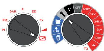
The Bluetooth® interface is set with the main rotary switch pointing to setting and the mode switch pointing at the remote control icon.
