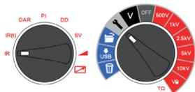
To set the clock and date, select the settings function (spanner) on the central rotary switch and turn the mode rotary switch to IR. Navigate using the left/right arrows to where the time and date is displayed.
