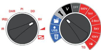
For a regular 5 step SV test, resistance readings for the first four 'steps' are displayed under consecutive time designators '1m' to '4m'. The 5 minute reading is displayed by the main display. The standard SV test duration can be adjusted if desired from the 5 minute default value using the up/down arrows and OK to save the setting. If the default 5 minute test duration is changed by the user the four readings will not show the respective '1m' to '4m' indicators.
