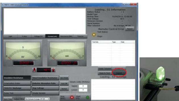
To activate the Import/Live Stream Control application click the Import soft button (circled) in the remote control application
