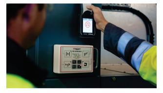
The box starts operating directly after being switched on, and generates partial discharge-like pulses. The level and frequency of the pulses, as well as the type of decoupling, are based on the current settings, which can be adjusted as following using the buttons on the front panel:
