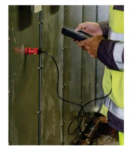
It is essential that this type of sensor is used correctly. The sensor head must be placed flush on a surface that is as smooth as possible. Even the smallest air inlets pose a risk of preventing signals caused by partial discharges from being measured.
