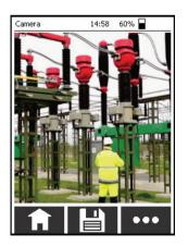
If the green cross indicating which can be enabled /disabled (see page 49) appears in the centre of the screen, it should be positioned as precisely as possible on the identified problem area or any other point relevant to the measurement when capturing the image. The green mark will then also be visible in the image file afterwards.
