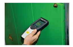
*Flexible* This external, acoustic sensor is specially designed for openings, air holes and gaps, *airborne acoustic* out of which the acoustic waves of the partial discharges can escape from the *sensor* switchgear.
