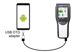
The measurement data stored in the internal memory of the PD Scan can then be easily and quickly shared via email, messaging or a cloud-based service using a compatible Android file management app.
