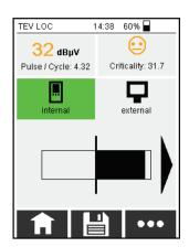
The black bar deflects in the direction of the sensor that is closer to the <u>weak point</u>. In the example, the weak point is considerably closer to the external sensor.
