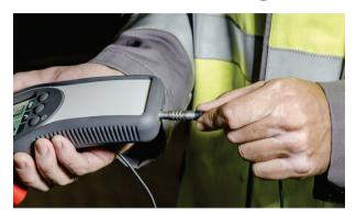
The device automatically detects the connected sensor after being switched on, and offers a choice between the potential operating modes.
