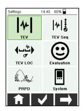
Along with the menus that are always available for editing device settings, the evaluation criteria and the PRPD diagram settings, the settings for the respective operating modes available (depending on the sensor connected) can also be entered.
