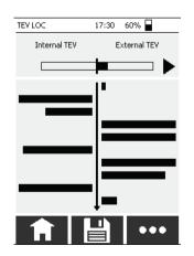
This screen allows you to monitor precisely how repositioning the sensors affects the measured levels.
