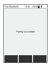
After being successfully paired for the first time, the headphones only have to be switched on after the PD Scan in future, and should then connect to it automatically. However, the 3 symbol only appears after an acoustic measurement was started.
