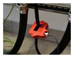
In principle, the PD Scan can also be used in combination with other HFCT couplers, as long as they feature an accessible BNC interface. However, depending on the sensor used, this may result in differences in the level display. The PD Scan has been precisely harmonised with the HFCT sensor in terms of its measurement accuracy.
