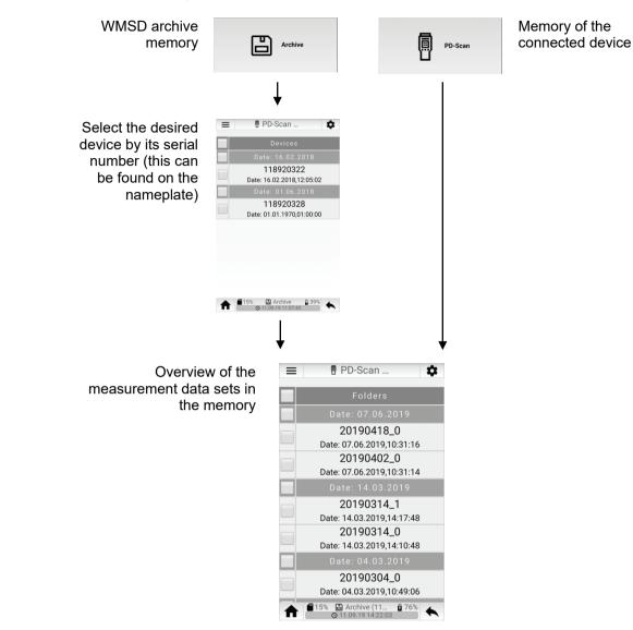
All measurement data stored in the memory of the connected PD Scan should also be stored in the archive database once the automatic data transfer is complete. However, the measurement data on the connected device can usually be located more quickly in the device's memory as it normally contains fewer data sets and the device does not need to be selected as described above.
