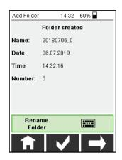
A new folder is created, the name of which is comprised of the current data and a running index.
