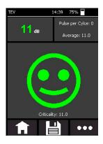
The user is also supported with the presentation of the measurement results. Measurement data is evaluated automatically, and feedback about the condition of the asset is provided visually by means of a smiley face and other ways. If the customer wishes other trending limits for the interpretation of the data, this can simply be individually customized.
