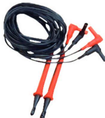
6 ft CAT IV 300 V rated compact kelvin probes, 4 mm shrouded plugs
