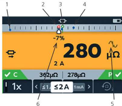
DLRO2 color display with new Difference Meter
