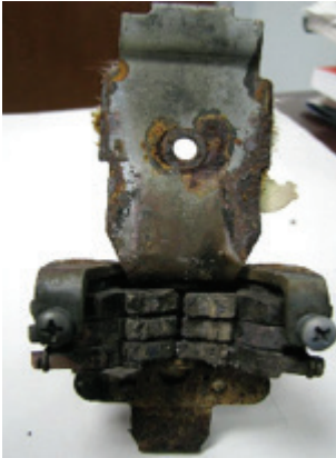
Fig 28: Circuit breaker corrosion
