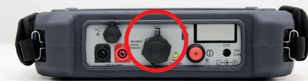
Connect the Duplex Kelvin Clips to the BITE5. This measurement can be made with the Duplex probes, however the Kelvin Clips may be easier.
