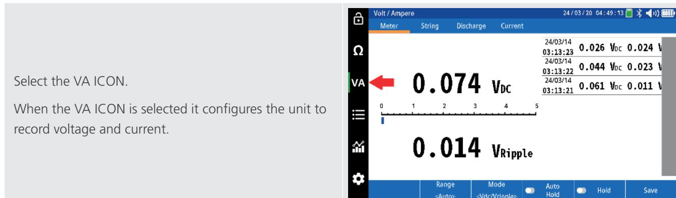
When the VA ICON is selected the BITE5 Advanced will use the banana jack inputs and the current clamp input. (if desired)
