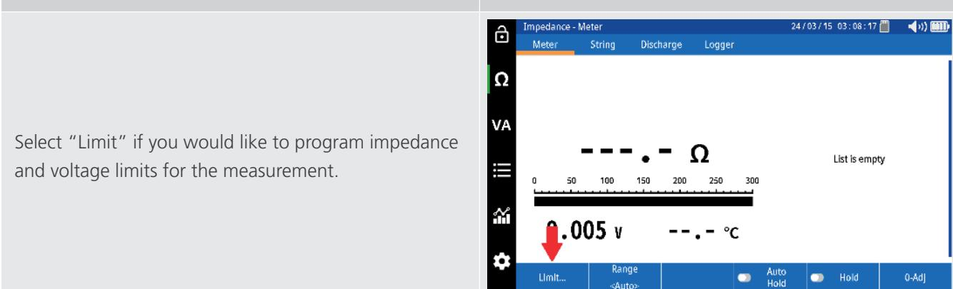
Select "Limit" if you would like to program impedance and voltage limits for the measurement.
