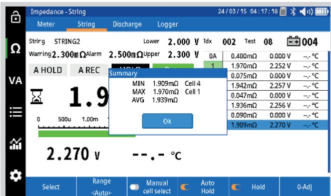
To record the negative terminal connection, close the summary and measure from the end of the negative charger lead to the last post on the last battery. This value will be saved as a strap.
