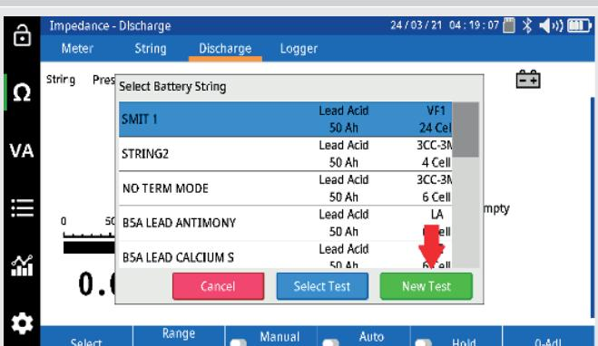
Start discharge test on load box. Take measurement of the first cell. The measurements will be saved with a date and time stamp.
