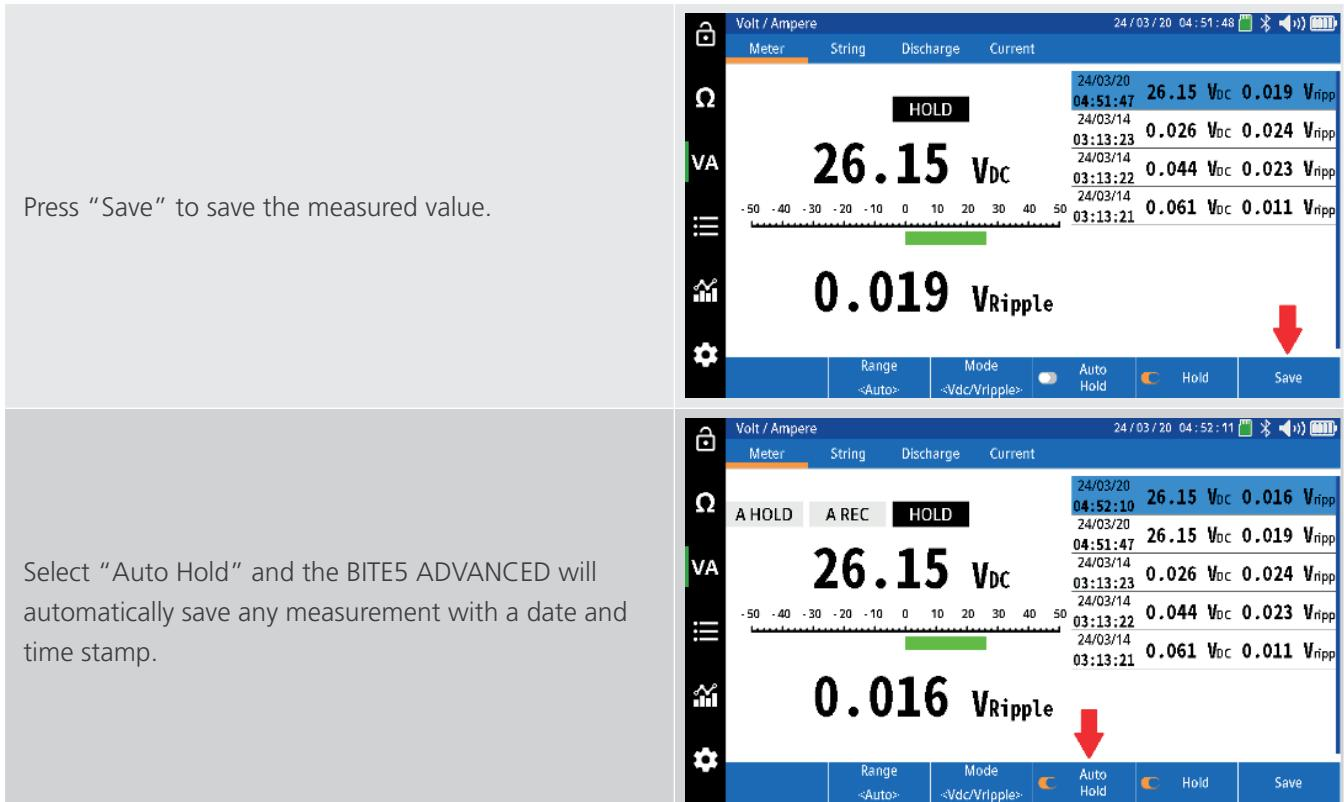
Adding a Ripple (AC) Voltage, Ripple (AC) Current or a Float (DC) Current value to a string.
