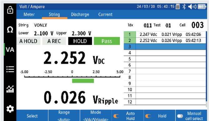
Continue through the string until the last cell is measured. At this point the BITE5 will display a summary of the test.
