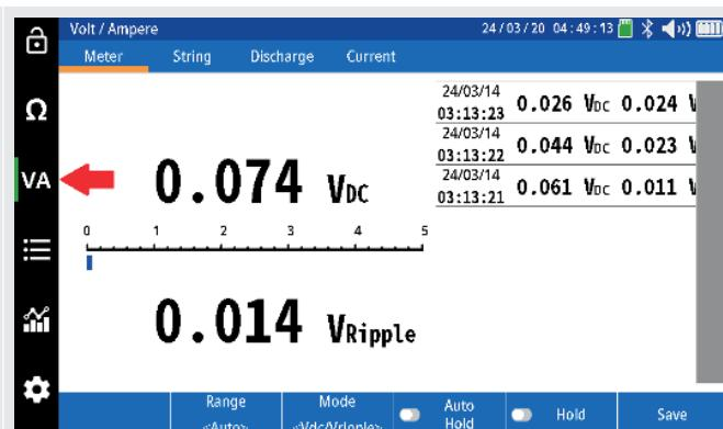
When the VA ICON is selected the BITE5 Advanced will use the banana jack inputs and the current clamp input. (if desired)
