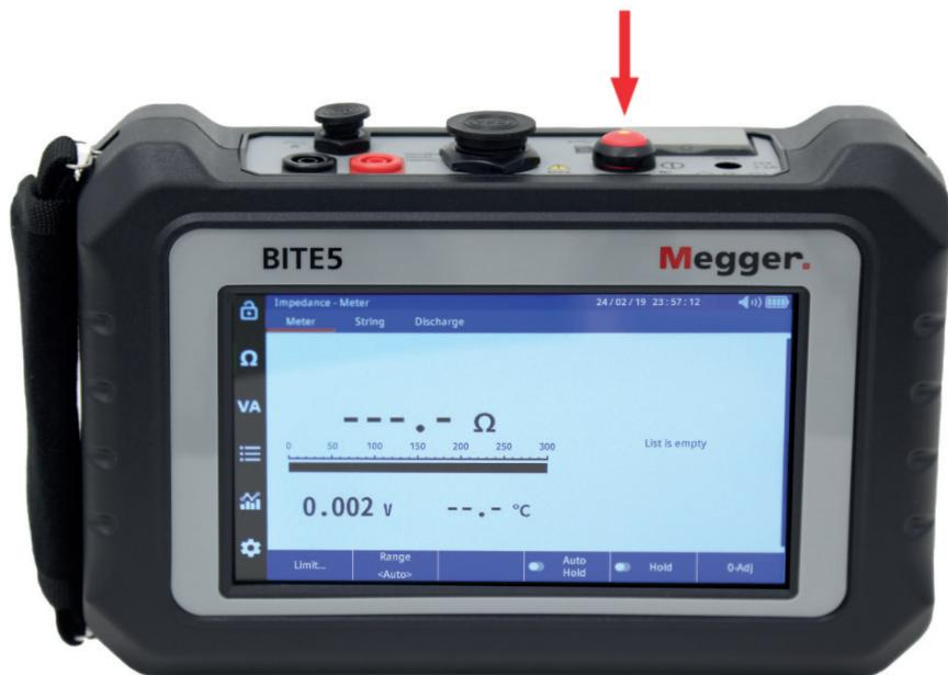
The displayed screen shall be saved to the SD card as a bitmap file. The bitmap will be located at the following path.
