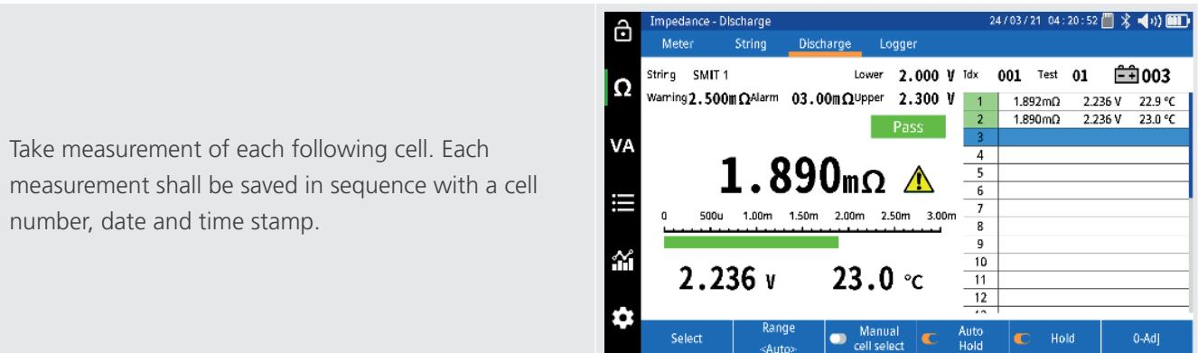
Take measurement of each following cell. Each measurement shall be saved in sequence with a cell number, date and time stamp.
