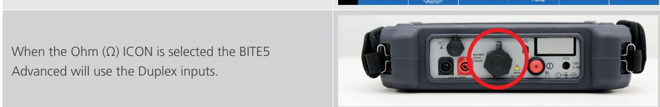
When the Ohm ( $\Omega$ ) ICON is selected the BITE5 Advanced will use the Duplex inputs.
