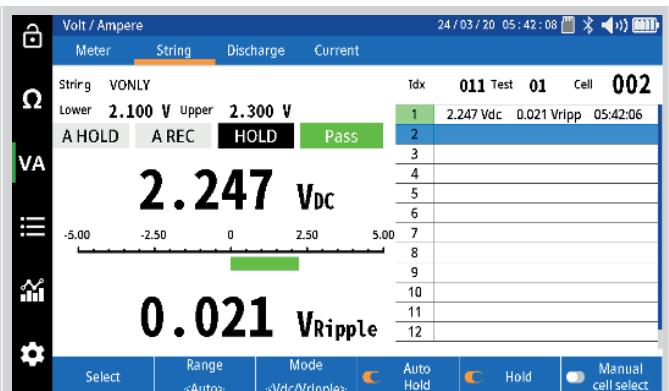
Proceed to the next cell. The BITE5 ADVANCED will automatically save and number the measured values.
